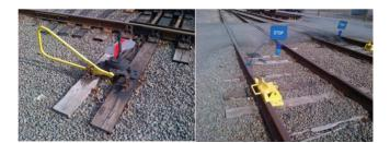
**6.0.9** Electrical power connection stations for rail equipment are located at the southern ends of each of VRE's yards and inside the equipment service and inspection building. This area presents tripping and electrocution hazards. Never step on or near the cables and do not handle them or any of the components associated with the power stations. If something appears wrong, notify the appropriate supervisor.
