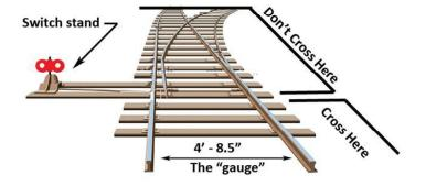
**6.0.4** Do not walk lengthwise between the two rails of a track (known as the "gauge" of the track) and *do not step on the actual rails.*
